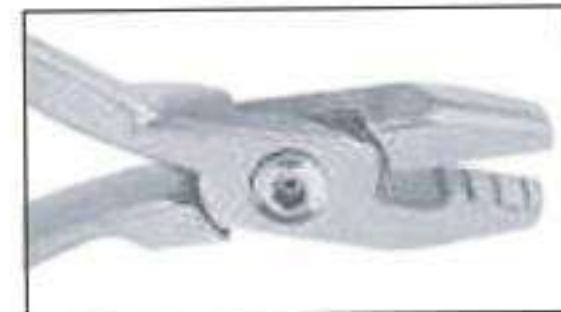
786-1391 Bending plier, in order to skirt molaras bands, with grooved Recommended wire .016", .018" and .022" .041mm, 0.46mm and 0.56mm
